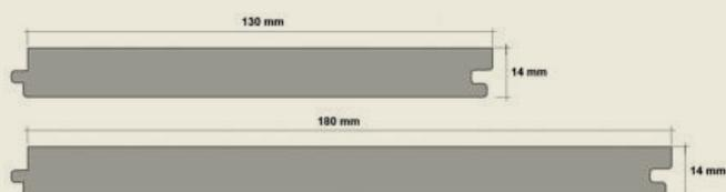
This gives the floor an equivalent wear layer to thicker flooring products and also increases the stability of the floor when under pressure from expansion. (see diagram below).
